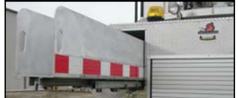
Optional Rear Blitz Line on Speedload Tray Holds up to 300' of 3" Double Jacket Fire
