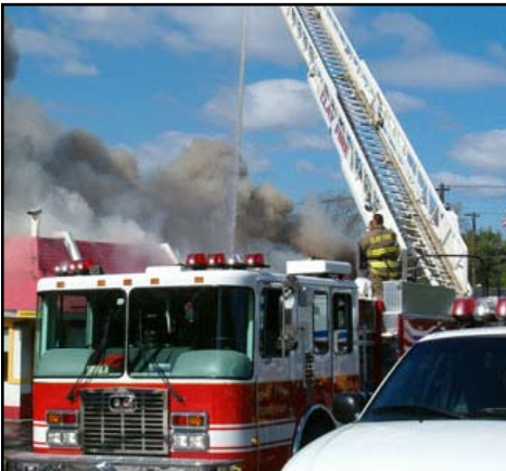
500 Pound Tip Load While Flowing 1000 GPM
