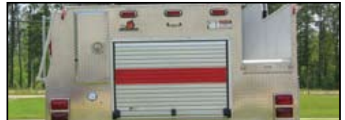
Enclosed Ladder Tunnel Holds 115' NFPA Ground Ladders and 6 Pike Poles
