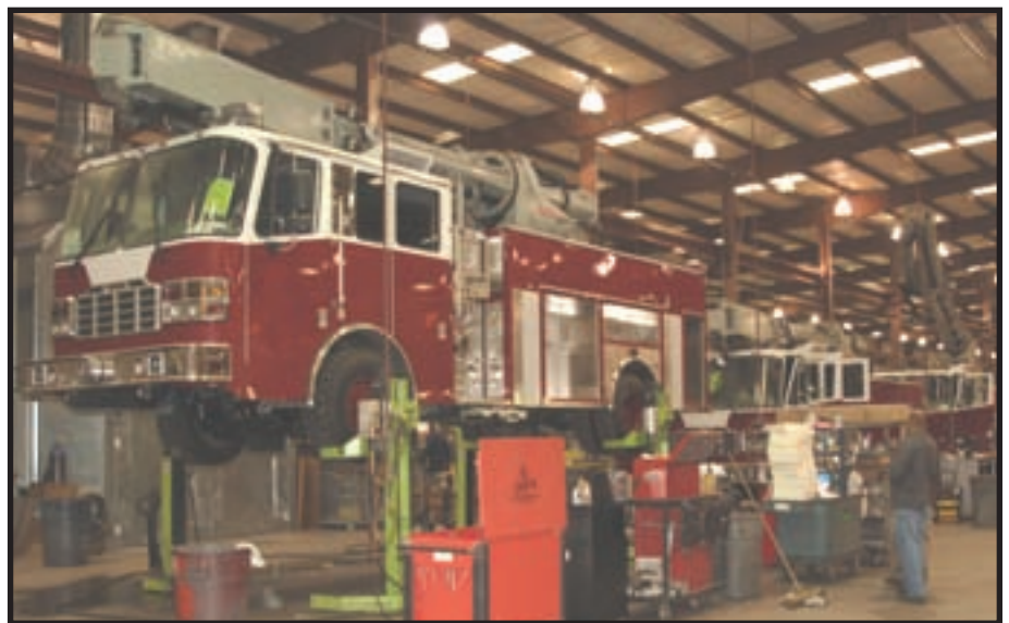
A Ferrara Strong Arm sits on a lift awaiting completion. Behind it are two additional units, part of an order of 10 for Istanbul, Turkey, ready to move down the line. The apparatus are built on Ferrara-built heavy-duty all-wheel drive cabs and chassis. By the beginning of the new year, the company expects to have 20 of the unique vehicles in service worldwide. (Fire Apparatus Photo by Jon Gilbert Fox)
