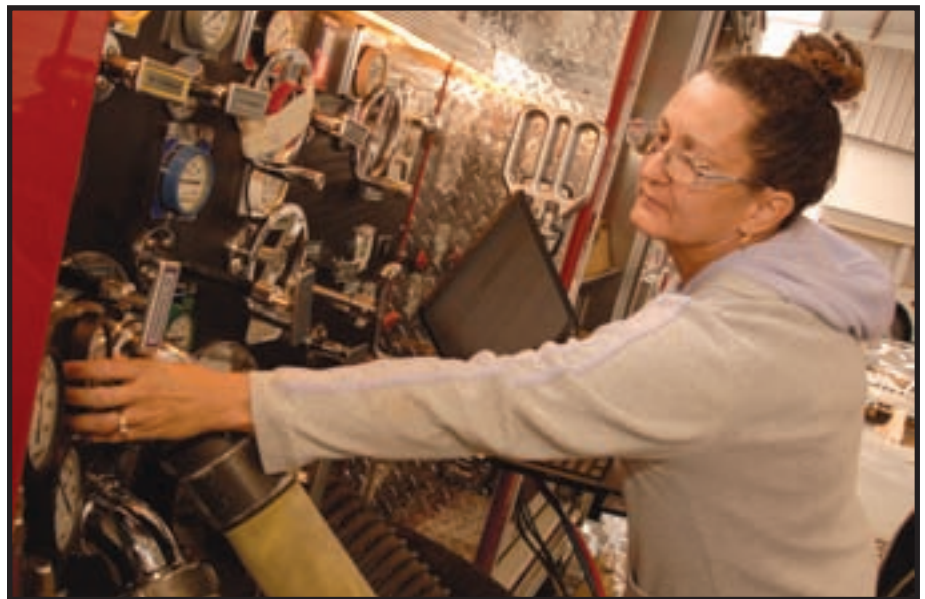
Felicia Sovinee, an Underwriters' Laboratories field inspector, tests a newly completed pumper for the Harvey (La.) Volunteer Fire Company. A UL field inspector is permanently assigned to the company, on site every day, putting apparatus through its paces. The company is on track to surpass 350 units completed in 2007. (Fire Apparatus Photo by Jon Gilbert Fox)
